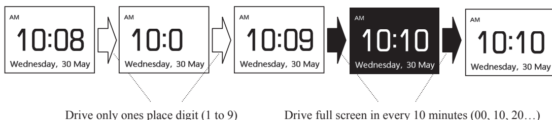
Fig. 8 Drive sequence of Cal.S770
