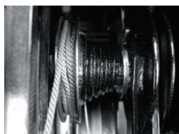
Fig.20 Wooden cone pulley in Arrow-shooting Boy
