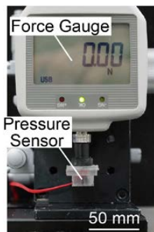
Fig. 7 Experimental setup for measuring the basic property of pressure sensor.
