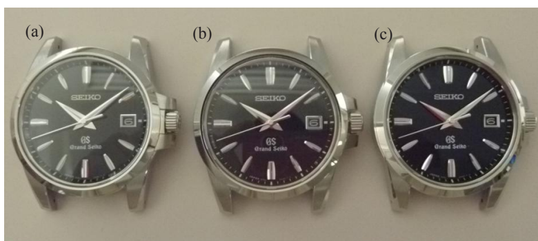
Fig. 2 Effect of Anti reflection coating. (a) Sapphire glass (no coating). (b) Back side anti reflection coating on sapphire glass. (c) Both side anti reflection coating on sapphire glass.
