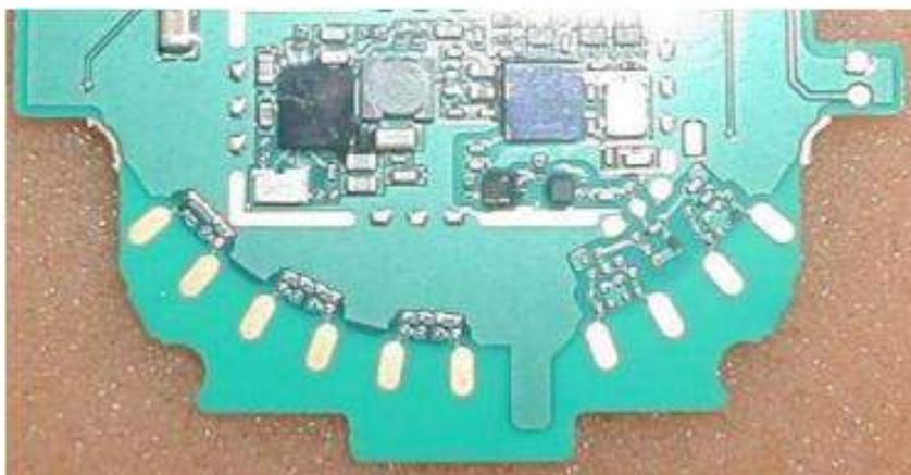
Fig. 8 Terminals on the circuit board to adjust the resonance frequency.
