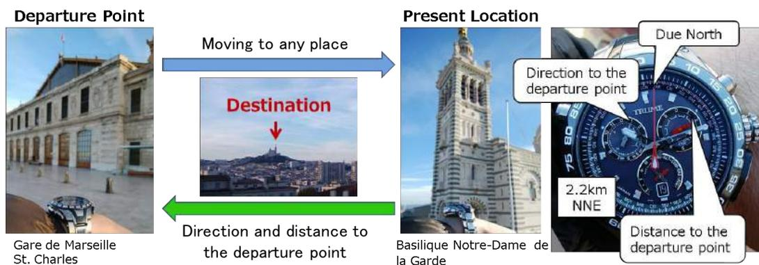
Fig. 2 Navigation function of TRUME MB8.
