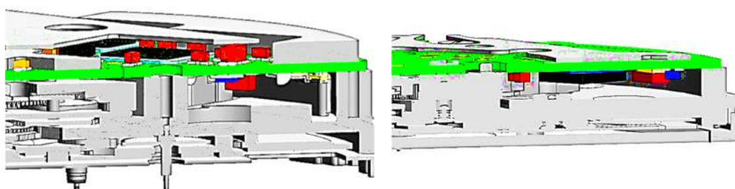
Fig. 7 Module thickness difference image in the component mounting. presence / absence of the back surface of the substrate. Presence / Absence
