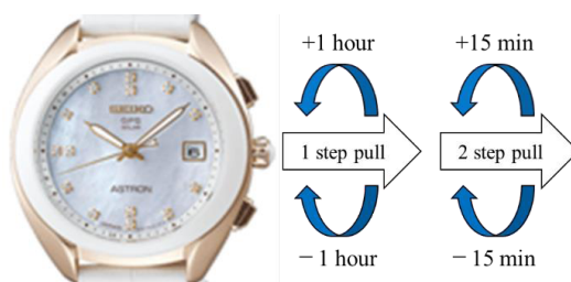
Fig. 19 Time adjustment of Cal. 3X.
