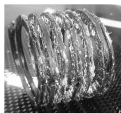
Fig. 10(c) CFRP coil spring (2×5) type UD. Fig. 10(d) CFRP coil spring (5×2) type UD.
