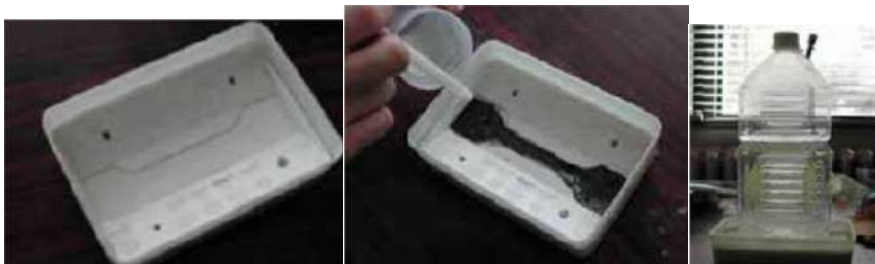
(a) Silicone rubber mold (b) Carbon fiber 3K cloth (c) 24 hours hold at 22°C
