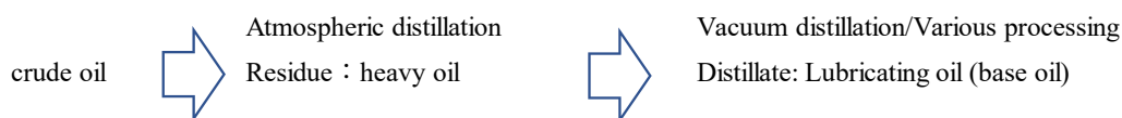
Fig. 2 Outline of the process from crude oil to extraction of lubricating base oil.
