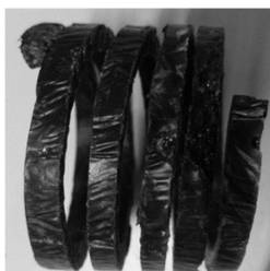
Fig. 10(a) CFRP coil spring (4×5) type UD. Fig. 10(b) CFRP coil spring (4×5) type UD/MAT.
