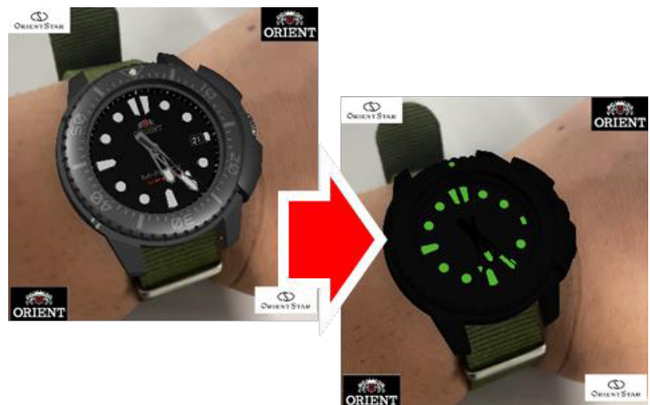
Fig. 12 Checking the luminous state of phosphorescent materials.
